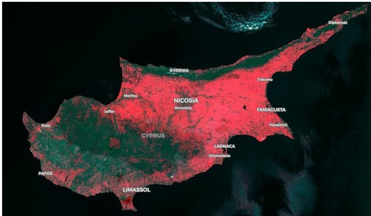
Figure 16: An overview of the bare-soil classifier over Cyprus, taken on 2020-05-13. The red color marks the detected bare soil (credit: European Union, contains modified Copernicus Sentinel data 2020, processed with EO browser).
