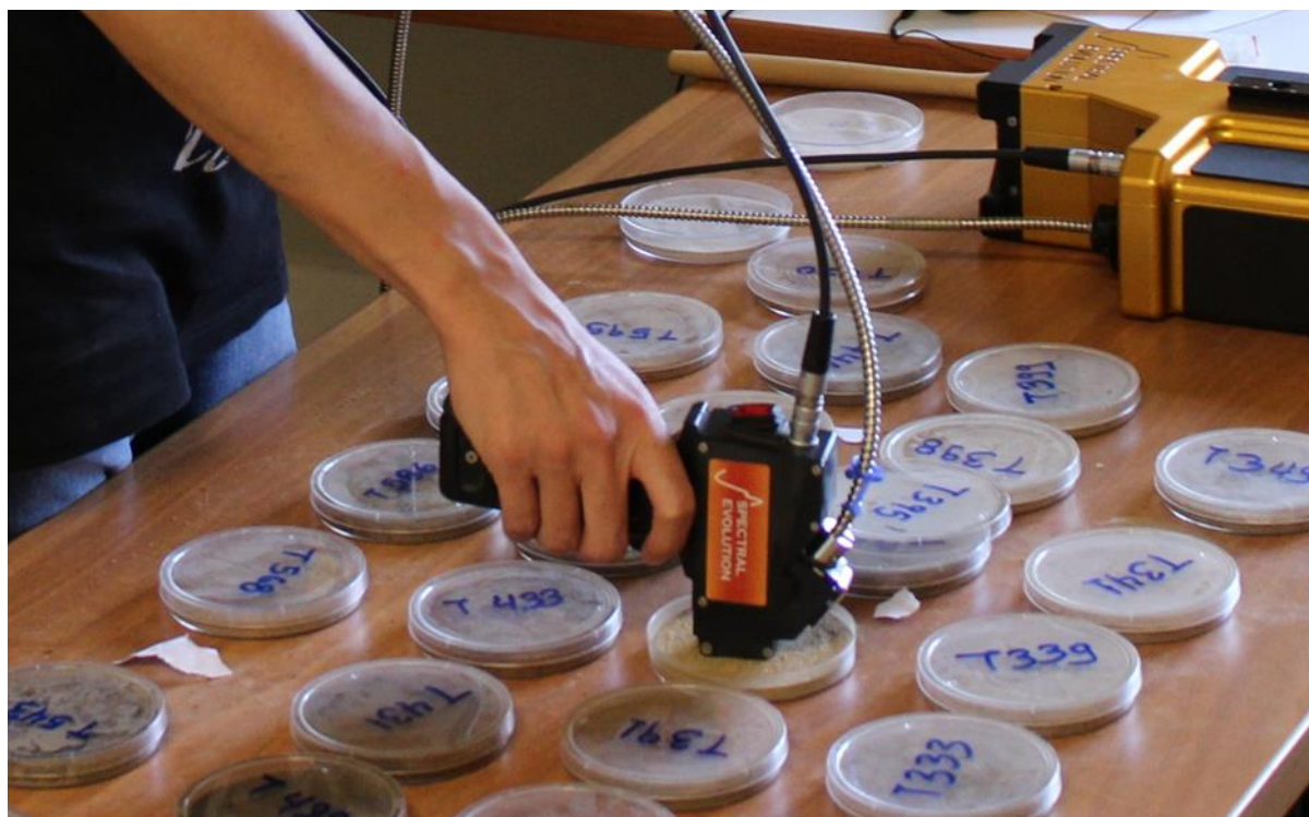
Figure 2: Measurement of diffuse reflectance spectroscopy in the laboratory using a contact probe bearing an optical fiber
